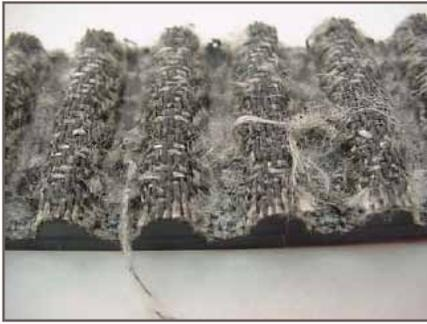
Figure 12 - Extreme tooth wear from worn sprockets
