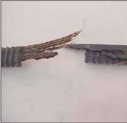
Figure 1 – Normal fatigue failure
