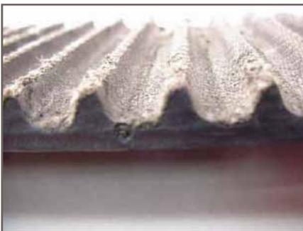
Figure 9 – Excessive tooth wear
