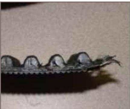
Figure 5 – Tooth root crack propagation
