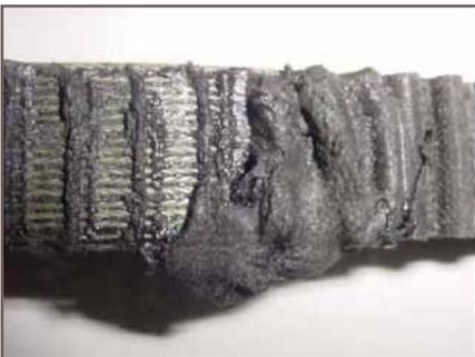
Figure 18 - Melting from high temperature operation, polyurethane
