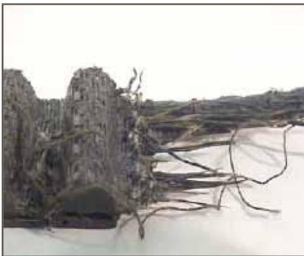
Figure 4 – Typical shock load failure
