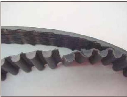
Figure 8 – Tooth separation failure
