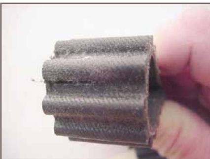
Figure 11 - Uneven belt wear
