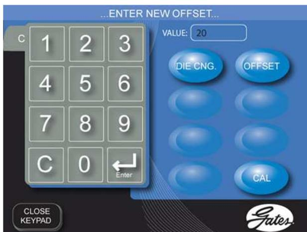
**CAL** – Allows access to Factory Calibration and is not necessary for normal operation of the GC96 crimper. **Strictly ONLY for USE by qualified Gates Maintenance Engineers.**
