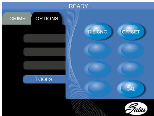
**DIE CNG** – Holding this button will automatically select head direction and move the head to a position more suitable for Standard GC32 Die Changes. It may be necessary to press the button twice to get it into the die change position.
