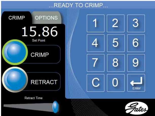
**RETRACT** – Pressing the retract button will cause the dies to open. This is a “Dead Man” control feature.
