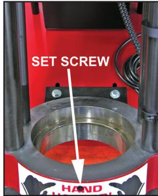
**1** Remove the standard Pressure Plate by loosening the set screw holding it in place. The set screw is located through the hole in the Hand Hazard Decal. A 1/8 inch hex key wrench is required.
