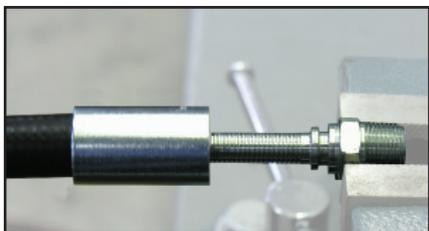
4. Lubricate the first two or three serrations on the stem with lightweight oil (SAE 10W)
