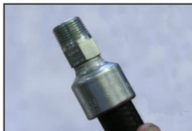
4. Insert coupling into the hose until the mark lines up with the end of the coupling ferrule.
