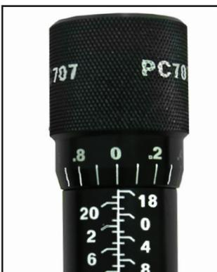
**7** Adjust the Dial Vernier to the setting obtained from the Gates Manual for the combination of hose and fitting being crimped.
