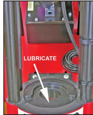
**3** Orient the Pressure Plate as shown and tighten the set screw to hold it securely in place. Lubricate the Pressure Plate with a high quality moly-disulfide grease. Molykote "G" is recommended.
