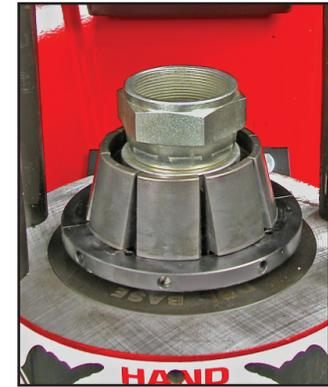
**5** Insert the Hose and fitting from the bottom of the crimper.
