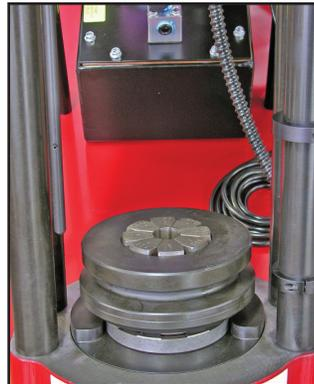
**5** Position the Compression Ring loosely over the die set and insert the hose and fitting from the bottom of the crimper.
