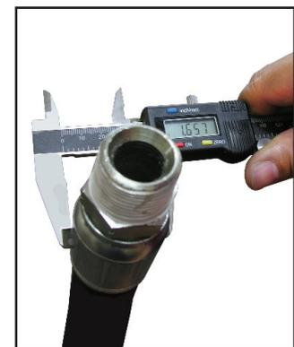
**8** Always measure the finished crimp diameter to be certain that it is within the Gates specification.
