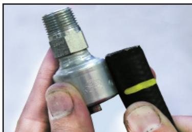
3. Place a visible mark on the hose cover at the insertion length shown in the crimp data manual.
