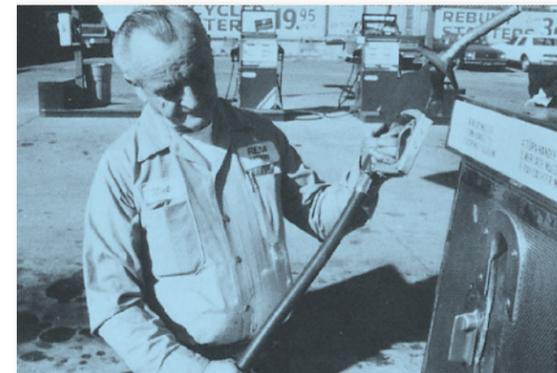
*Inspect hose cover for cracks or cuts.*
