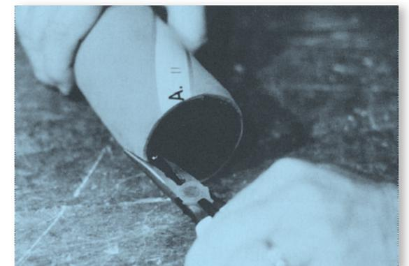
*Pinching the staple into the tube wall.*
