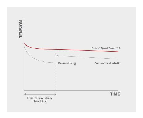
By using innovative minimal-stretch cord technology, Gates® has designed the industry's first bandless zero-maintenance V-belt.
