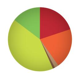
**Improper Drive Maintenance 42% Improper Installation 20% Poor Design 20% Environmental Factors 15% Improper Handling 2% Defective Components 1%**
