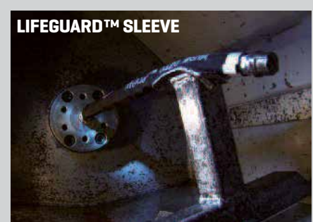
LIFEGUARD™ SLEEVE The LifeGuard™ sleeve contained and effectively redirected fluid during 10,000 psi (68.9 MPa) burst tests while hoses without sleeving exploded, releasing a large amount of fluid in the immediate area.
