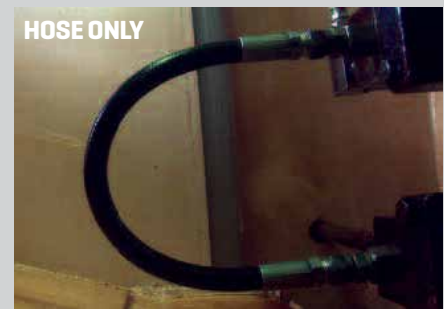
LIFEGUARD™ SLEEVE During 5,000 psi [34.5 MPa] pinhole leak tests, LifeGuard™ sleeving controlled and redirected fluid while unsleeved hoses allowed high-pressure spraying of fluids in the immediate vicinity of the leak.
