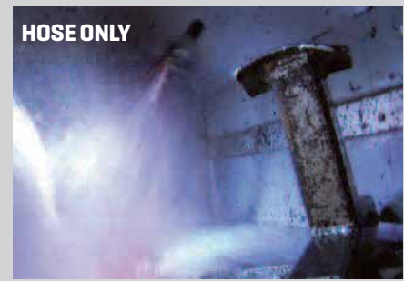
LIFEGUARD™ SLEEVE The LifeGuard™ sleeve contained and effectively redirected fluid during 10,000 psi (68.9 MPa) burst tests while hoses without sleeving exploded, releasing a large amount of fluid in the immediate area.
