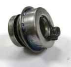
To the right are examples of Dynamic and Static seal contamination/ filming /caused by over use of sealants. When sealant particulates / residue get trapped between the Dynamic and Static seal faces it causes a separation of the two surfaces which leads to a seal leak.
