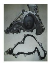
In the examples below one can see where sealer material has been found within the cartridge seal and has led to premature leakage of the water pump and the customer returned the pumps as an alleged manufacturer defect.
