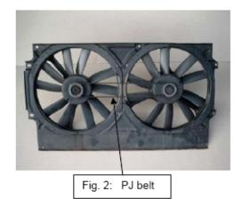
In cases where additional cooling is needed, such as cars with air conditioning, factory installed tow bar, for taxis etc., a second fan is installed in order to pull more cooling air through the radiator. This second fan is then often driven from the first by a 2 or 3 rib PJ belt.
