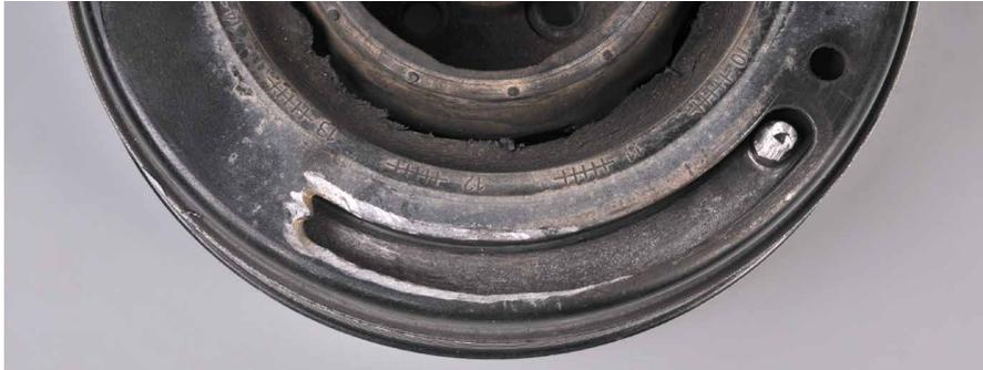
Only for those types of torsional vibration dampers that have wear indicating tabs which allow checking the angular displacement of the rubber versus the pulley.
