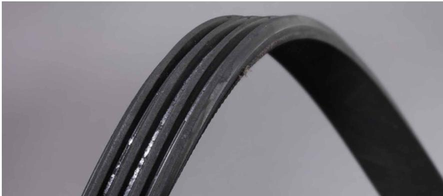
**Appearance:** Belt material wears off from the ribs and builds up in the belt grooves.
