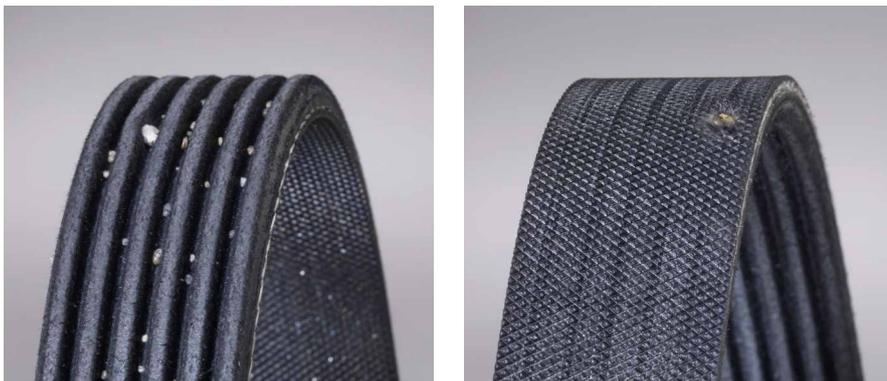
**Appearance:** Small pinholes are visible on the backside of the belt. Bumps may be visible and fabric around the holes can be frayed.
