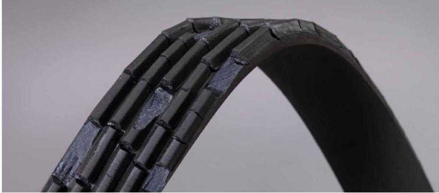
**Appearance:** Pieces or chunks of rubber material have come off the belt. When chunk-out has occurred, a belt can fail at any moment.
