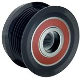
Every time the engine decelerates, for example during gear changing or engine shutdown, the alternator's inertia creates resistance against the belt. An overrunning alternator pulley allows the alternator to "free-wheel" or "overrun" when the belt suddenly slows down. This prevents the belt from slipping and reduces vibration, wear and chirp noises.
