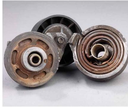
**Appearance:** Rust is bleeding between arm and base or dripping from the tensioner. Also, check the tensioner for cracks or damage to arm, housing and bracket. Some damage can't be seen unless the tensioner has been removed.
