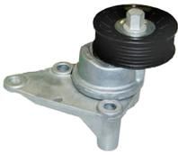
The vast majority of vehicles using a multi-ribbed belt have an automatic belt tensioner. Tension is provided by a powerful spring, located within a small canister-like housing to which a pulley is attached. The pulley pivots around the spring housing and generates a constant belt tension. Automatic belt tensioners are designed into the belt drive system for several reasons:
