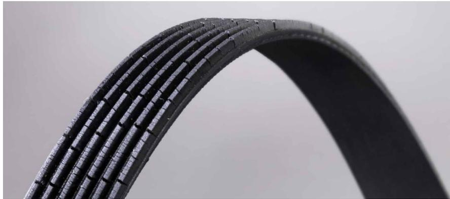
**Appearance:** Small yet visible cracks along the length of a rib or ribs.
