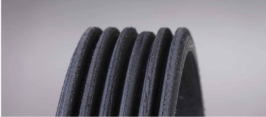
**Appearance:** Wear that is more severe on one rib than on the others or one rib that exhibits a different wear pattern than the others. A thumping or grinding noise may also be heard.
