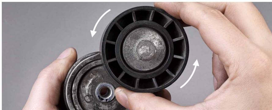
**Appearance:** With the engine off and the belt removed, manually rotate the pulley. If you notice noise, resistance or roughness, the problem is likely to be pulley bearing wear.
