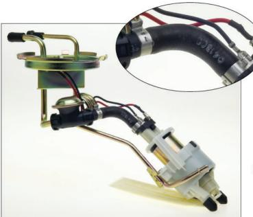
Unfortunately, too many in-tank fuel pump repairs improperly use ordinary fuel line hose for the pump-to-valve connection
