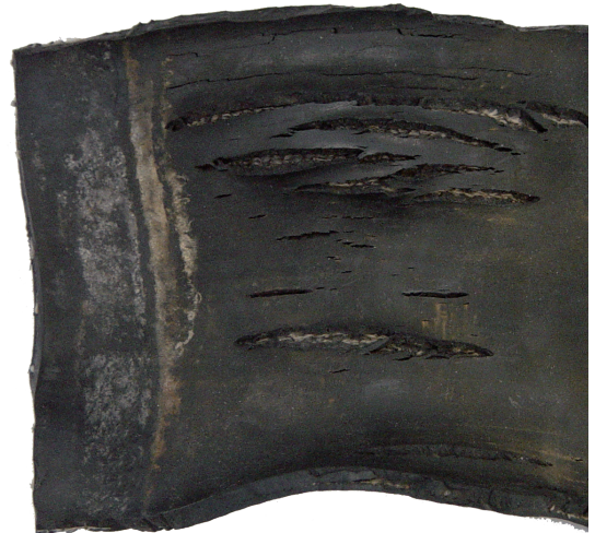
An example of coolant hose failure caused by ECD.
