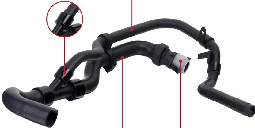
In addition, a lot of modular hoses have sensors, flow restrictors and directional valves inside of them that can get damaged
