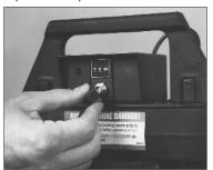
• Loosen the two (2) set screws in the brass knob 1/4 to 1/2 turn using a .05" Allen wrench.
