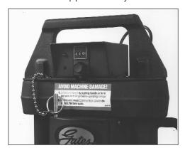
Turn pump on by pressing and holding the power "on" switch, (see pump operating manual for switch location) which extends the ram.
