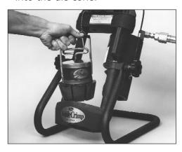
Remove magnet by lifting the "T" handle, making sure the top of the die fingers are even.
