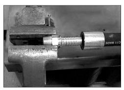
Hose should be flush against stem shoulder (see cutaway drawing below).
