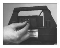
Note: Rotating the knob on front of switch box clockwise will increase the number; counterclockwise will decrease the number. When changing the setting, always move to a highter number then down to the desired setting. (Example: To change from 200 to 245, move dial up to 300 then down to 245.)
