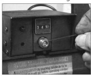
• Turn the brass knob either clockwise or counterclockwise to get the setting back to 245.
