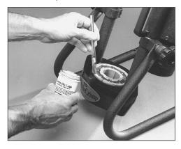
\* Use only Gates Molykote lube for proper operation or Gates-recommended grease.
