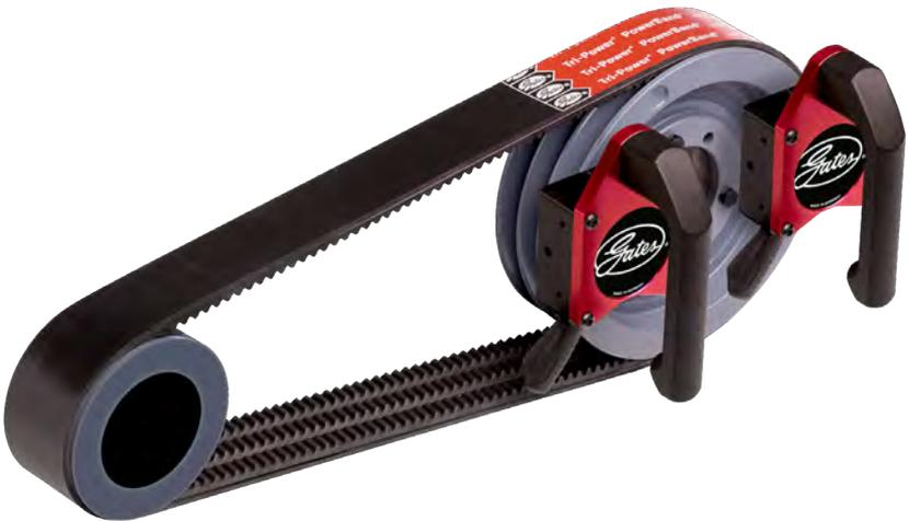
5. Rotate the magnetic clamp activation lever by 60° into the “ON” position. Always check to make sure the lever springs into the locking notch.
