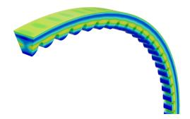
Moulding notches into the belt helps reduce and spread out these stresses.
