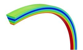
Using Finite Element Analysis (FEA), the increased bending stresses are clearly visible on a belt without notches.
