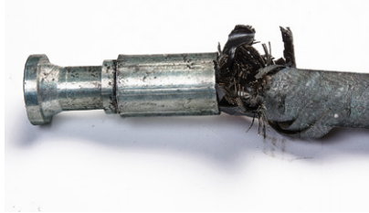
Hose Burst at Coupling
