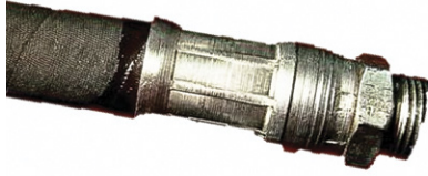
Weep at Hose/Coupling Interface
