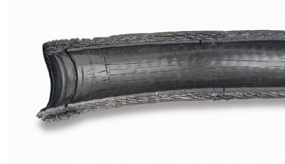
Hose Tube Failure
