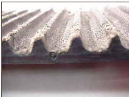
Figure 9 – Excessive tooth wear
