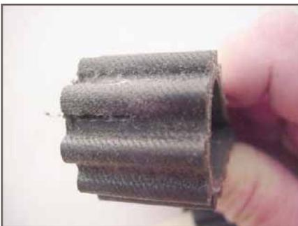
Figure 11 - Uneven belt wear
