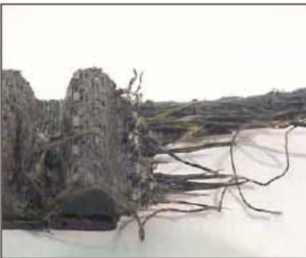
Figure 4 – Typical shock load failure
