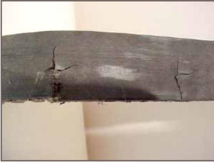
Figure 19 - Tensile cord failure from debris
