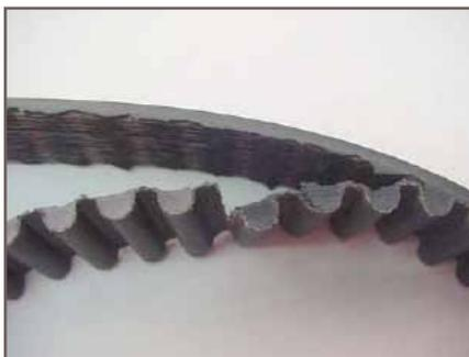
Figure 8 – Tooth separation failure
