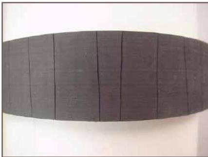
Figure 17 - Cracking from high temperature operation, rubber
