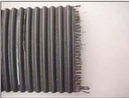
Figure 20 - Crimp failure due to debris
