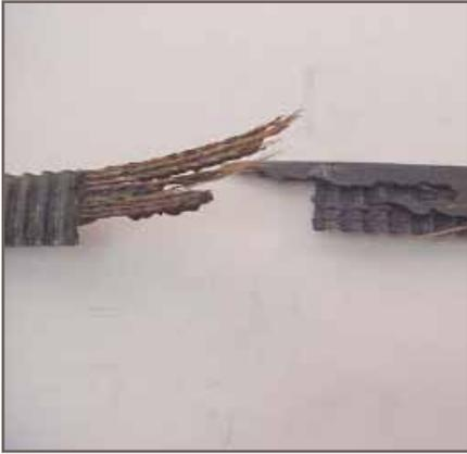
Figure 1 – Normal fatigue failure
