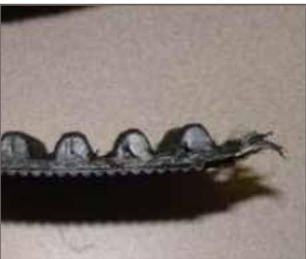
Figure 5 – Tooth root crack propagation
