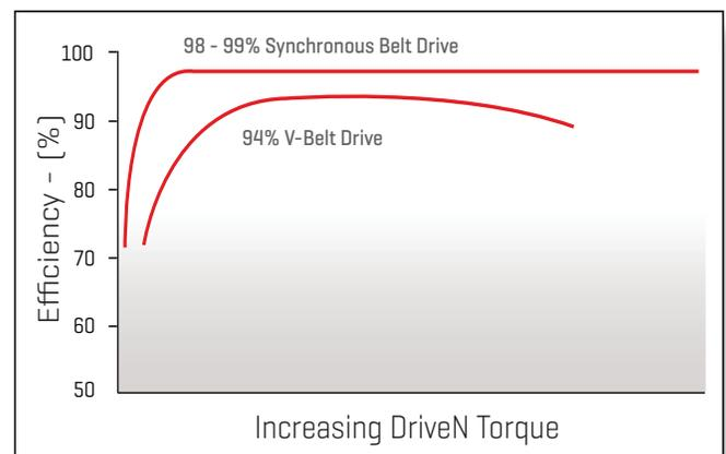
*On average, a synchronous belt drive is 5% more efficient than a standard V-belt drive, eliminating excess energy consumption.*
