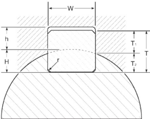
Figure 2: Keyway and Key Size
