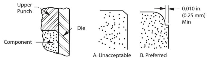
The radius of the corner in example (A) cannot be pressed because it would require a feather edge on the punch. The edge may be relieved with a flat edge as seen in example (B).
