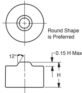
A boss can be formed in the punch face at either end of the component provided that the guidelines for the draft and height are observed.
