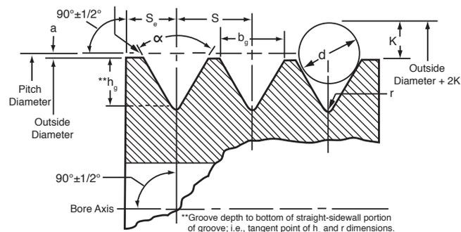
Figure 8 - Polyflex Sheave Groove Dimensions
