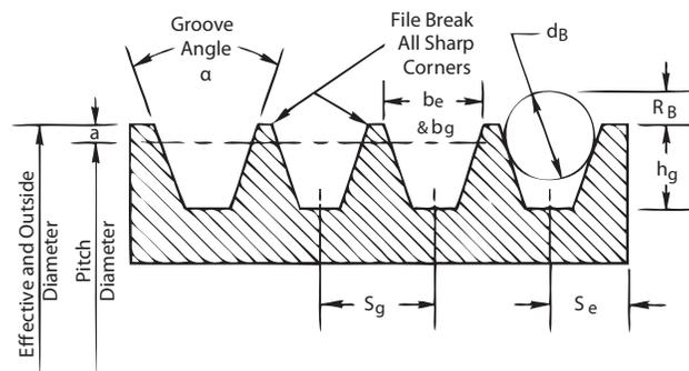
Figure 4 - Sheave Groove Dimensions
