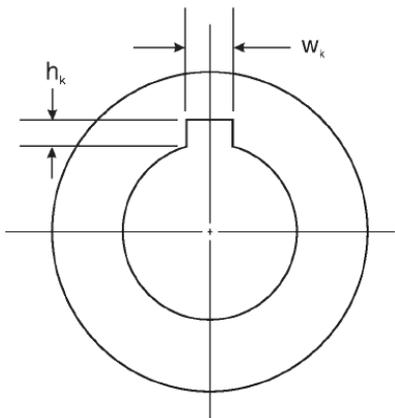
Figure 9- Sprocket Profile
