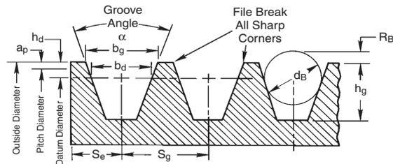
Figure 3 - Groove Dimensions (for tables 12 and 13)
