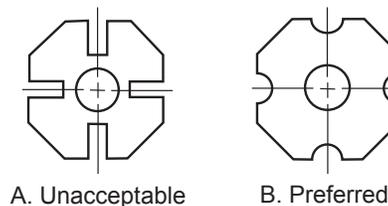
The design of (A) requires long, thin tool membranes, and the sharp corners cause problems in powder fill. Design (B) avoids both problems.
