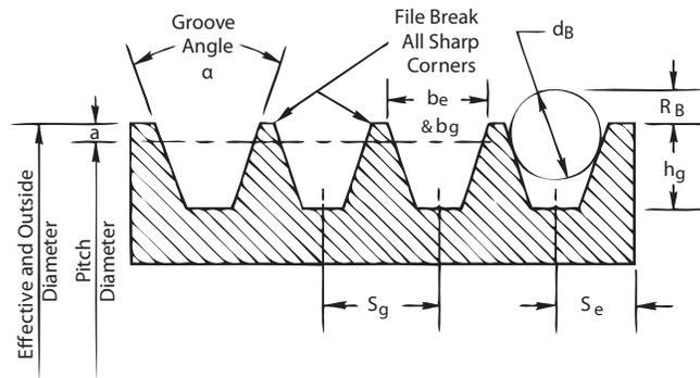
Figure 7 - Metric Sheave Groove Dimensions
