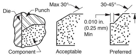
A chamber is preferred to a radius at the intersection of tool members. Angles 30° or less from radial provide sufficient tool strength. Angles 30-45° should terminate in a flat. Angles greater than 45° should be avoided.
