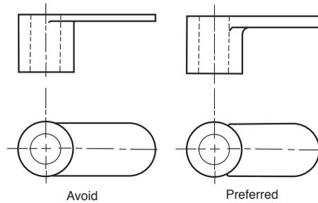
Large, thin protrusions should be as thick as permissible and be joined to more massive features with generous radii.
