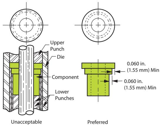
Multiple steps require a minimum 0.060 in. (1.5mm) axial difference to allow adequate strength in the punches.
