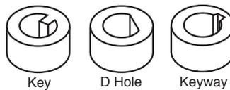
Keys, D holes, and keyways can be formed in hubs in the compaction operation.
