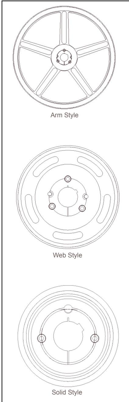
Figure 1 - Common Styles of Sprockets and Sheaves
