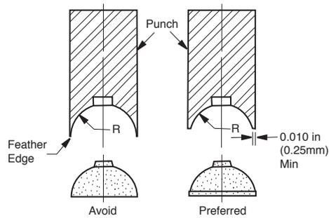
A flat on the diameter of the sphere allows the punch to terminate a flat rather than a feather edge.
