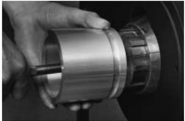
**C.** Pull the die fingers out of the die shoes approximately 1/2", then position the die can over the end of the die fingers and pull them into the die can.
