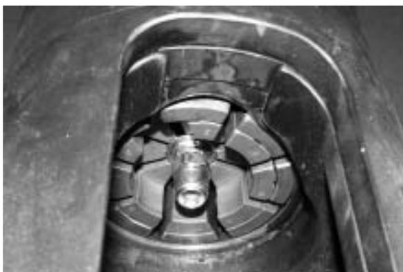
9. To start the crimp cycle, press and release the START CRIMP switch. As soon as the die fingers contact the ferrule, pull slightly on the hose assembly. This will ensure that the ferrule locking collar is properly located over the stem locking groove. The crimper will extend to the displayed CRIMP position and return to the RETRACT position.
