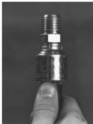
4. Insert coupling into the hose until the mark lines up with the end of the coupling ferrule.
