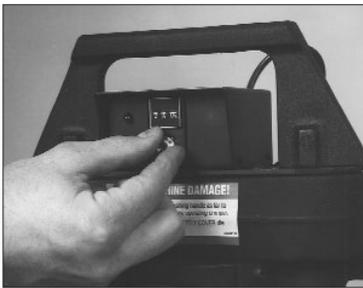
*Note: Rotating the knob on front of switch box clockwise will increase the number; counterclockwise will decrease the number. When changing the setting, always move to a higher number then down to the desired setting. (Example: To change from 200 to 245, move dial up to 300 then down to 245.)*
