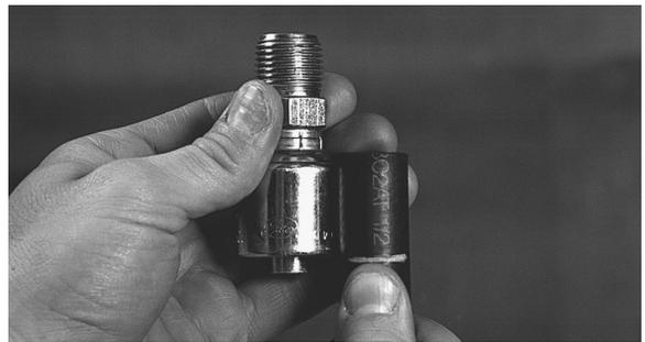
4. Insert coupling into hose until the mark lines up with coupling ferrule end.
