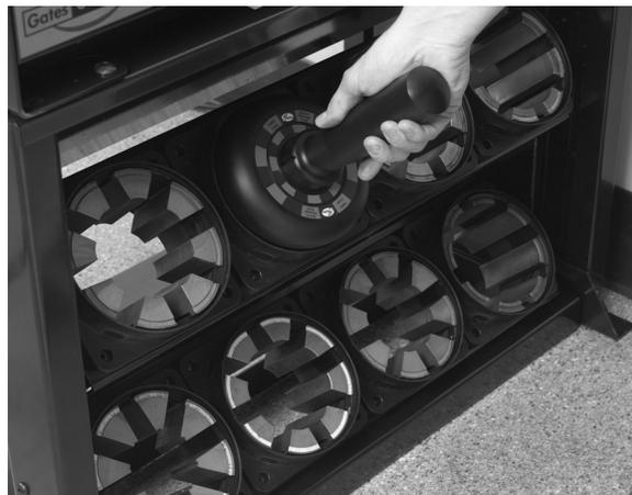
Turn power switch off. Using grease gun, grease both front (8) and back (16) die shoe grease fittings until grease appears between die and die cone surface (approximately 1 1/2 pumps). Fully cycle crimper 5 times to distribute grease evenly (alternate between top blue CRIMP button and bottom yellow RETRACT button, or actuate with foot pedal).
