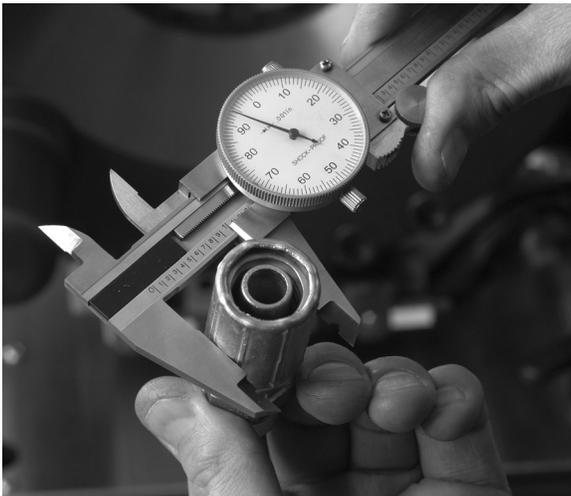
Crimp new assembly following steps 1-9 until proper crimp diameter is achieved.
