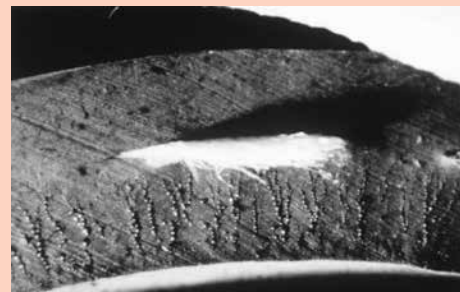
Tube cracking due to electrochemical degradation.
