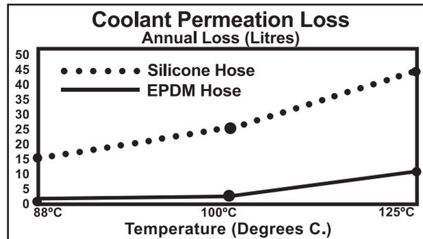
of water each year if it were equipped with silicone hose. The same truck equipped with electrochemical-resistant EPDM coolant hose would lose only one litre in the same period.
