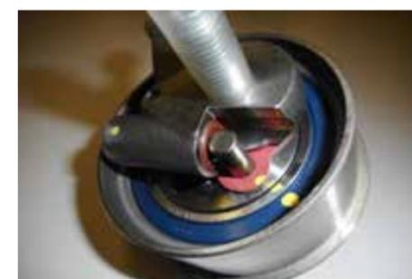
This is the correct state of the tensioner before installation.
