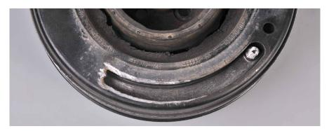
Only for those types of torsional vibration dampers that have wear indicating tabs which allow checking the angular displacement of the rubber versus the pulley.
