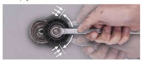
**Appearance:** Move the tensioner arm (tensioner being mounted on the engine) through its entire range of motion with a wrench. There should be resistance to this movement. If there is none, the spring has lost its force. Other indicators are belt squeal from slippage, or loss of rotation of a belt-driven component.
