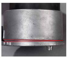
**Appearance:** Abnormal belt tracking on tensioner pulley. Shiny, smooth streaks or gouges in tensioner housing or arm.
