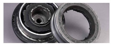
**Appearance:** The torsional vibration damper physically falls apart. It can also come off the engine completely, resulting in an immediate breakdown and collateral damage.
