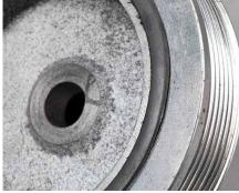
**Appearance:** The ring of elastomeric material is clearly deformed. The deformation initially becomes visible on the rear side of the damper. This kind of damage is frequently overlooked in inspections because the pulley itself is often not removed for visual inspection purposes and is only examined from the front.
