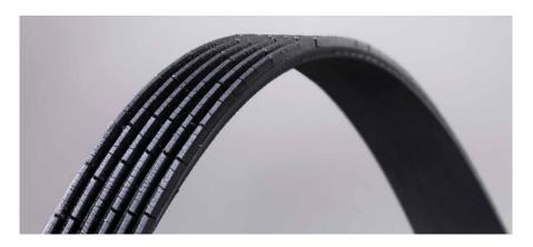
**Appearance:** Small yet visible cracks along the length of a rib or ribs.
