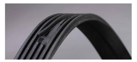
**Appearance:** A belt rib shears off or begins to separate from the belt base.
