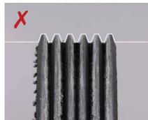
Gates ABDS (Accessory Belt Drive System) wear indicator helps you assess wear on EPDM belts and pulleys and determine when a belt or a pulley has lost so much material it negatively affects its performance and should be replaced. The tool is simple to use and allows you to quickly gauge wear – either on the engine or off.
