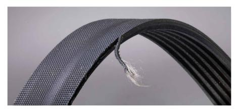
**Appearance:**Sidewalls of the belt may appear glazed or the edge-cord may become frayed and ribs removed. A noticeable noise may result. In severe cases, the belt can get pulled into the timing belt drive causing catastrophic engine damage.
