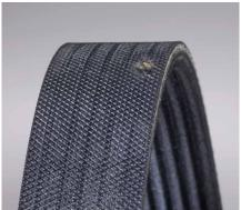
**Appearance:** Small pinholes are visible on the backside of the belt. Bumps may be visible and fabric around the holes can be frayed.
