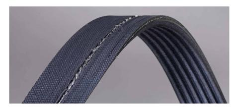
**Appearance:** Backside of belt appears shiny or glazed. In advanced stages, the fabric or even the cord becomes exposed and gets damaged.
