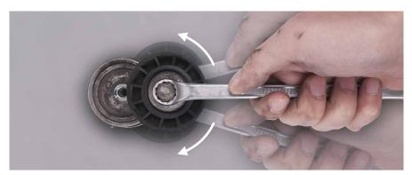
**Appearance:** Cycle the tensioner (mounted on the engine) through the entire range of motion (from stop to stop) by applying torque to the arm with a wrench. The tensioner arm should move smoothly and freely.
