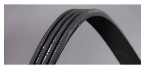
**Appearance:** Belt material wears off from the ribs and builds up in the belt grooves.
