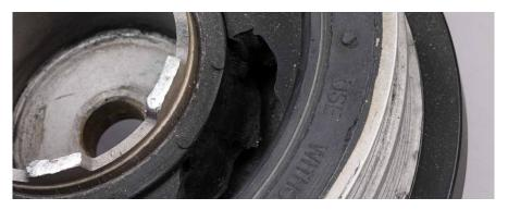
Appearance: The rubber loosens and gets stuck between the pulleys and the belt.
