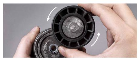
**Appearance:** With the engine off and the belt removed, manually rotate the pulley. If you notice noise, resistance or roughness, the problem is likely to be pulley bearing wear.
