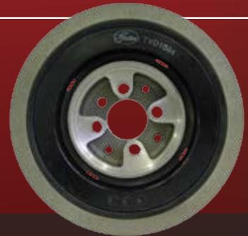
After a certain period of time, the harsh working conditions will inevitably start affecting the dampening device as well. The torsional vibration damper can break; deformation, wear and hardening can occur; the rubber can loosen, crack, get stuck between the pulleys or wear out; the outer ring can start slipping and even separate from the rest, or the damper can come off your engine completely!
