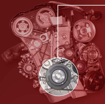
The crankshaft torsional vibration damper, a device which is mounted on the front end of the engine's crankshaft, is designed to reduce this twisting motion, therefore increasing engine component life and minimising crankshaft failure.
