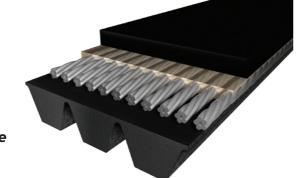
On the surface, Stretch-Fit belts may look like standard Micro V belts, but inside they are dramatically different. The secret is in Gates' new Twistlock technology, where the strength and flexibility of the advanced polyamide tensile cord is surrounded by a specially formulated adhesive that literally locks on to the cord allowing it to elongate and stretch but never lose tension.
