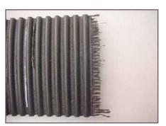
Figure 20 - Crimp failure due to debris
