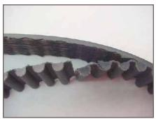
Figure 8 - Tooth separation failure
