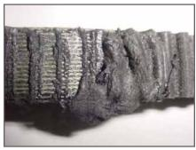
Figure 18 - Melting from high temperature operation, polyurethane
