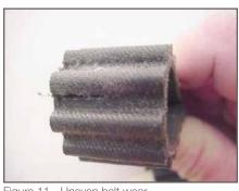
Figure 11 - Uneven belt wear
