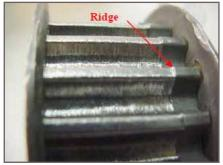
Figure 14 - Excessive sprocket wear
