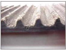
Figure 9 – Excessive tooth wear
