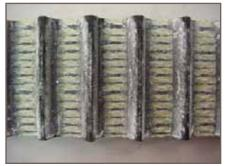
Figure 16 - Extreme wear from abrasion
