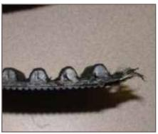
Figure 5 – Tooth root crack propagation
