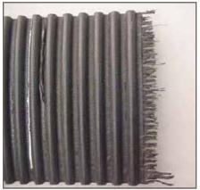
Figure 3 – Crimp failure
