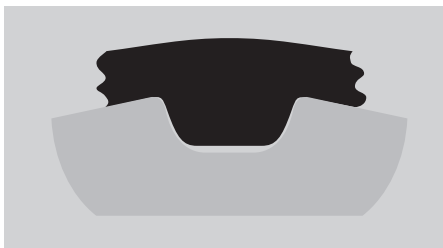
PowerGrip® Timing Belt Tooth/Groove Contact
