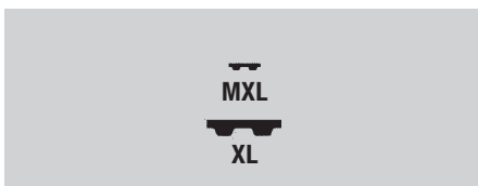
PowerGrip® Timing Belt Profiles/Pitches
