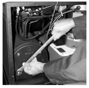
**G.** Crimp a –12PC1FS ferrule to check adjustment. If crimp diameter is not acceptable, repeat adjustment steps. If crimp diameter is acceptable, plug in cooling fan and replace back cover.
