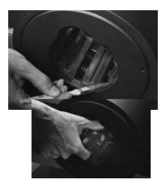
**C.** Using a small brush, apply a light coat of Molykote "G" grease to the sliding surfaces of both front and rear cones. Be sure to brush lube between the die shoes, but do not get lube on the shoes themselves. Rotate the die shoes by hand to spread the lube under them.
