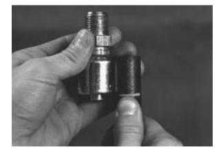
**3.** Place a visible mark on hose cover at the insertion length shown in the crimp data manual.
