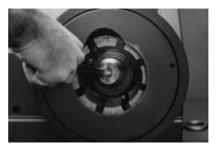
**A.** For dies larger than number 37, insert speed loader through the front of the crimper and beyond the die fingers. Jog the ram to the LOAD/UNLOAD position. Be careful not to crush loader head or handle by keeping handle centered in die.
