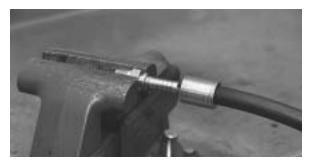
**4.** Lubricate the first two or three serrations on stem with lightweight oil (SAE 10W).
