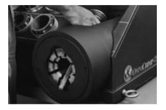
**B.** For dies 37 and smaller, insert the speed loader into the crimper through the opening in the main tube and position the loader handle out through the die fingers. Jog the ram to the LOAD/UNLOAD position. Be careful not to crush the loader head or handle by keeping handle centered in die.
