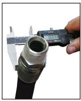
**9** Always measure the finished crimp diameter to be certain that it is within the Gates specification.
