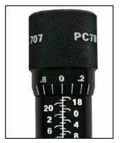
**7** Adjust the Dial Vernier to the setting obtained from the Gates Manual for the combination of hose and fitting being crimped.
