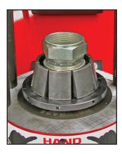
5 Insert the Hose and fitting from the bottom of the crimper.
