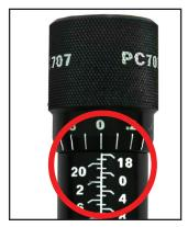
6 Adjust the Dial Vernier to the setting obtained from the Gates Manual. Note that for Double Angle Dies settings greater than 16 are above the zero due to the special calibration factors for Double Angle Dies.
