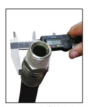
**8** Always measure the finished crimp diameter to be certain that it is within the Gates specification.
