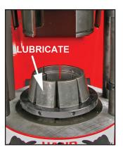
**3** Select the correct Double Angle Die for the hose and fitting combination being crimped. Lubricate the I D of the Bottom Base Ring and the top Compression Ring with a high quality moly-disulfide grease . Molykote "G" is recommended.
