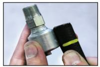
**3.** Place a visible mark on the hose cover at the insertion length shown in the crimp data manual.
