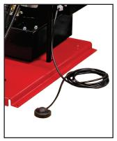
**8** Press and hold the pneumatic start/ stop switch until the motor shuts off and the ram retracts.
