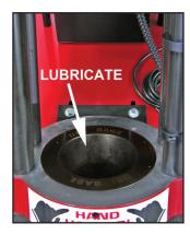
**2** Install the Double Angle Base Ring making certain that the bottom flange is clean and free of debris and that the base ring seats firmly and squarely in the bottom flange.
