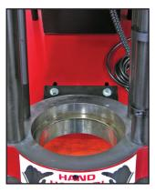
**2** Make certain that the base is clean. Insert the standard Pressure Plate and tighten the set screw through the hole in the hand hazard decal with a 1/8 inch hex key wrench.
