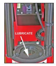
**3** Orient the Pressure Plate as shown and tighten the set screw to hold it securely in place. Lubricate the Pressure Plate with a high quality moly-disulfide grease. Molykote "G" is recommended.
