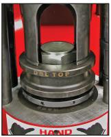
**7** Install the Pusher on the ram if it has been removed and press and hold the pneumatic start/stop switch until the motor shuts off and the ram retracts.
