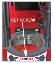
**1** Remove the standard Pressure Plate by loosening the set screw holding it in place. The set screw is located through the hole in the Hand Hazard Decal. A 1/8 inch hex key wrench is required.
