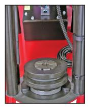
**5** Position the Compression Ring loosely over the die set and insert the hose and fitting from the bottom of the crimper.
