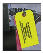
**1** Note the tag attached to the pump motor and make certain that the power source matches the requirements specified on the tag.
