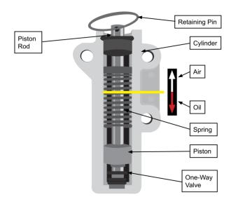
Due to normal shipping and handling procedures, there exists a strong possibility that air has entered the fluid chamber of the included tensioner. Therefore, one **MUST** complete the following bleed procedure prior to hydraulic tensioner installation.
