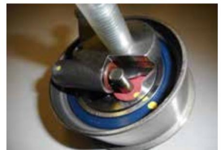
This is the correct state of the tensioner before installation. **DO NOT** install if the tensioner assembly does not resemble the image above.
