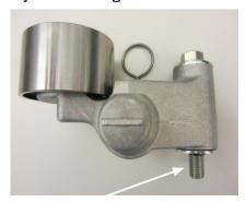
Apply Threadlocker to tensioner pivot bolt threads prior to installation.
