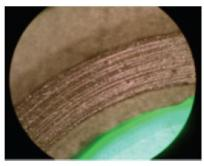
Contamination causing scratches on seal ring surface.
