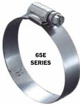
Lined clamps are specially designed for use with silicone rubber and other soft hose applications. The liner protects the hose surface and prevents it from extruding or shearing through the band notches as the clamp is tightened.
