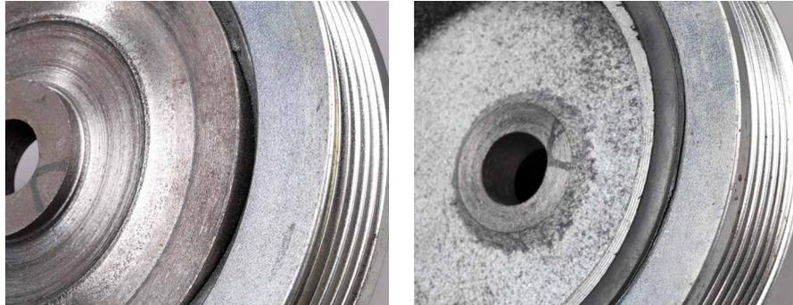
**Appearance:** The ring of elastomeric material is clearly deformed. The deformation initially becomes visible on the rear side of the damper. This kind of damage is frequently overlooked in inspections because the pulley itself is often not removed for visual inspection purposes and is only examined from the front.
