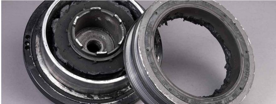
**Appearance:** The torsional vibration damper physically falls apart. It can also come off the engine completely, resulting in an immediate breakdown and collateral damage.
