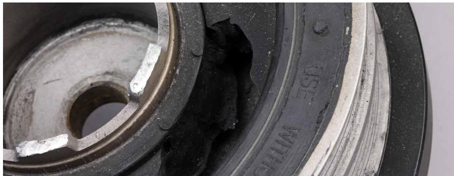
**Appearance:** The rubber loosens and gets stuck between the pulleys and the belt.
