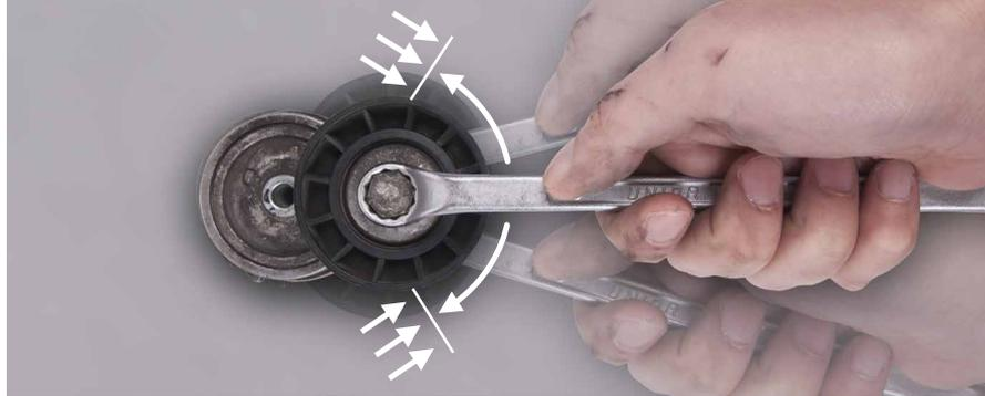
**Appearance:** Move the tensioner arm (tensioner being mounted on the engine) through its entire range of motion with a wrench. There should be resistance to this movement. If there is none, the spring has lost its force. Other indicators are belt squeal from slippage, or loss of rotation of a belt-driven component.
