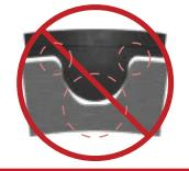
The belt tooth is too large to fully seat in the sprocket groove
